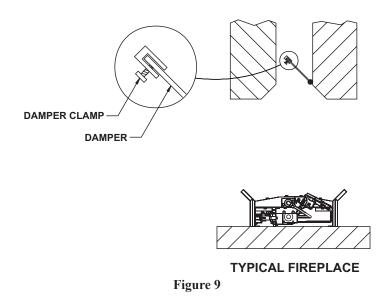
When installing your log set as a vent-free installation the damper clamp can be used to eliminate the potential for odors when burning the logs for the first time.
